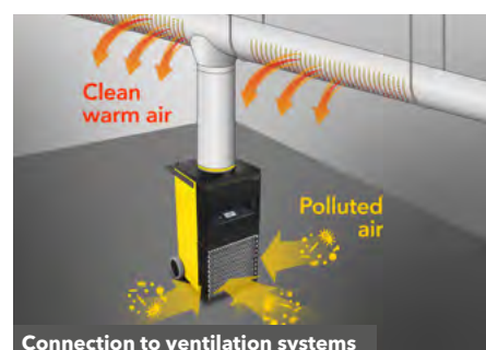
Connection to ventilation systems
